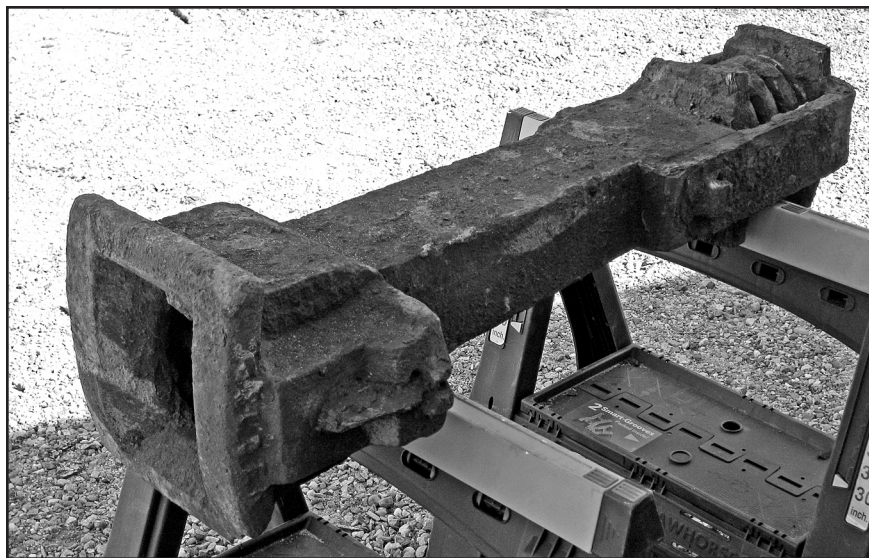
The recovered late 1880s Master Car Builders design link-and-pin coupler. – Photo © 2012 Norm Acker.
